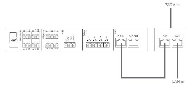
Alternatively the TanGo can be connected to a PoE enabled switch:
